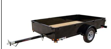
This 6×10 ft single axle trailer is compact and versatile, with steel sides and tailgate to securely haul an ATV or other cargo, and tilt for easy load and unload. It's available with an optional 4 wood sides at 20" high or 3 wood sides at 11" high above the metal sides, which are easily removable. Every Chilton Trailer is built by hand with a fully welded frame and ramp for years of reliability.
