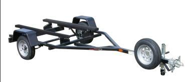
This single place personal watercraft trailer (approx. 6x13 ft) is light and easy to tow, with a 1285 lb carrying capacity and an optional swivel jack with wheel. Every Chilton Trailer is built by hand with a fully welded frame for years of reliability.
