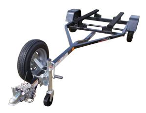
Model PW52-15-2 shown with optional spare tire and adjustable swivel jack with wheel.
