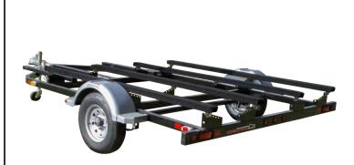
This two place personal watercraft trailer (approx. 8.5x15 ft) is light and easy to tow, with a 2549 lb carrying capacity and a standard swivel jack with wheel. Every Chilton Trailer is built by hand with a fully welded frame for years of reliability.
