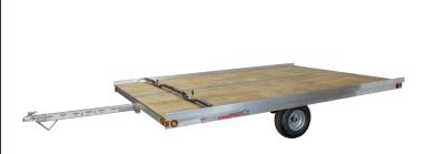
This single axle 8.5×10 ft snow trailer is light and easy to tow, with room for 2 snowmobiles, and tilt or a slide-out rear ramp option for easy loading. Every Chilton Trailer is built by hand with a fully welded frame for years of reliability.
