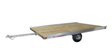
This single axle 8.5×10 ft deckover trailer is light and versatile, with room to haul anything from an RC or riding mower to building materials, with standard tilt or slide-out ramp options for easy loading. Every Chilton Trailer is built by hand with a fully welded frame for years of reliability.
