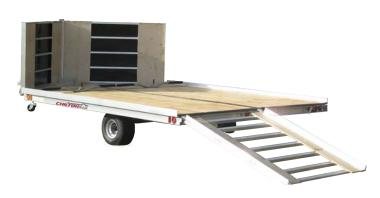
Model SD22-12A2-EZA shown with optional salt shield / drive off ramp package.
