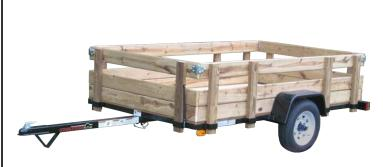
This 5x8 ft single axle trailer is light and versatile, with tilt for easy loading. It's available with optional wood sides at 20" high or 11" high, which are easily removed. Every Chilton Trailer is built by hand with a fully welded frame for years of reliability.
