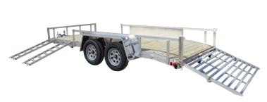
This 7×17 ft heavy-duty tandem trailer easily hauls your ATV and UTV, with a 2 ft beavertail and side-load ramps conveniently integrated into the load retaining rail. Both the standard straight rear ramp and optional bi-fold ramp fold down flat on the trailer deck for easy hauling when empty. Every Chilton Trailer is built by hand with a fully welded frame and ramps for years of reliability.
