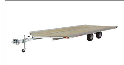
This tandem axle 8.5×20 ft v-front snow trailer is light and easy to tow, with room for up to 4 snowmobiles. Every Chilton Trailer is built by hand with a fully welded frame and ramp for years of reliability.
