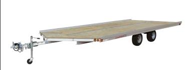
This tandem axle 8.5x20 ft v-front deckover trailer is light and versatile, with room to haul anything from building materials to an RC or riding mower. Every Chilton Trailer is built by hand with a fully welded frame and ramp for years of reliability.
